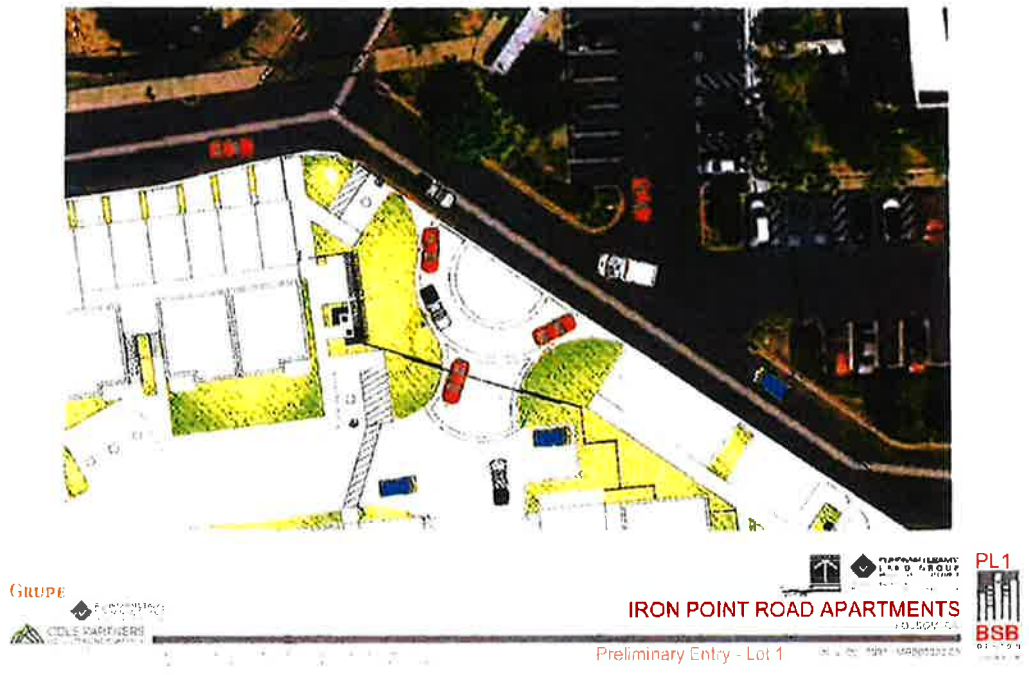
Figure 3. Entry Gate Detail At For "Lot 1" (Western Portion Of Project) Showing Queue Storage At Entry Gate
