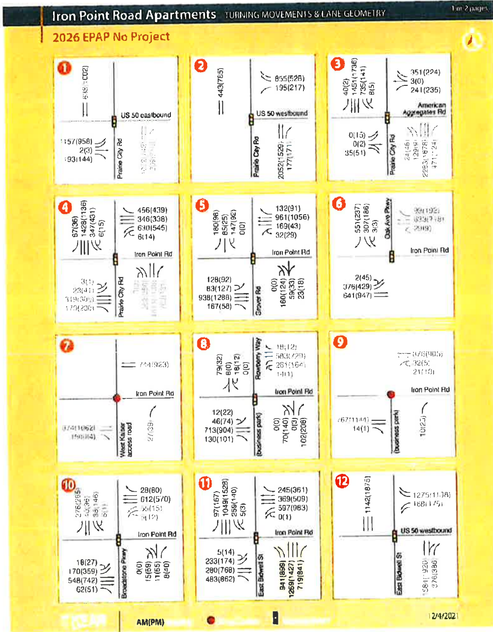
Figure 17. EPAP 2026 Condition Turn Movements and Geometry
